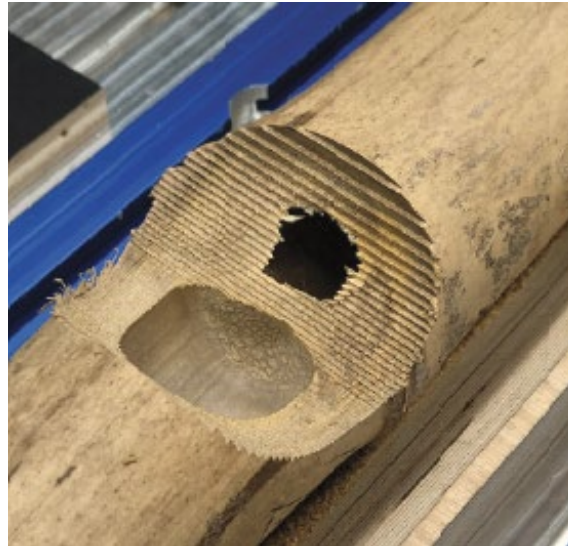
Figure 4 Example of bamboo member milled at node
