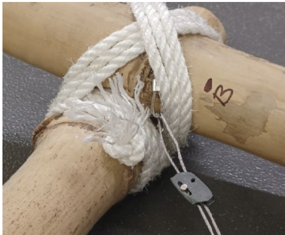
Figure 6 Tensioning and lashing a reciprocal unit
