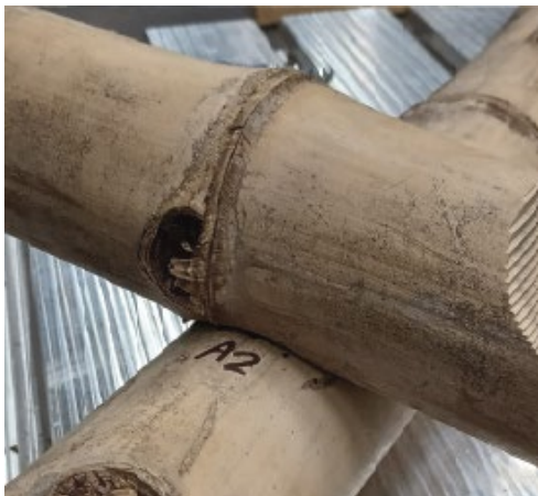
Figure 3 Example of members pairing and labelling
